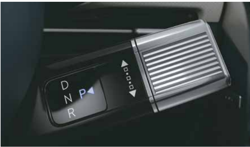
Shift by wire (SBW Column type)
